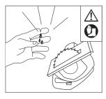
Blade and sharp burrs which could cut hands. Wear protective gloves and keep a safe distance from the cutting area.
