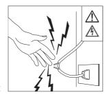
Risk of electric shock and danger of death. Do not touch the electrically live parts and keep a safe distance. Before any maintenance operations, unplug the machine from the power supply.
