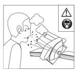
Material and dust flying towards the operator's eyes and body. Use eye protection and an antidust mask.
