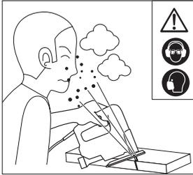
Material and dust flying towards the operator's eyes and body. Always wear eye protection and an anti-dust mask.
