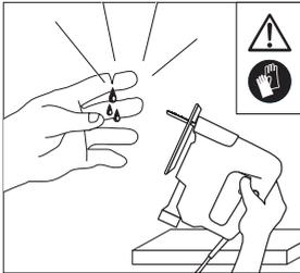
Blade and splinters/burrs that cause hand injuries. Wear safety gloves and keep a safe distance from the cutting area.
