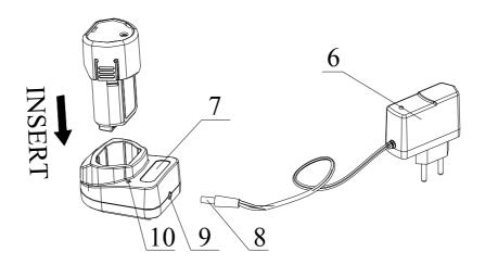
◆ Plug the mains plug of the adaptor 6 into a socket outlet and the adaptor plug 8 into the socket 7 on the charger station 9. At this time, the battery charge-control indicator 10 lights up. And then insert the battery pack into the charger station. The battery charge-control indicator indicates the charging progress. The indicator lights up red during the charge procedure. The battery is completely charged when the indicator lights up green again.
