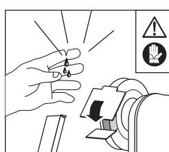
Moving parts and sharp burrs which could cut hands. Wear protective gloves and keep a safe distance from the grinding area.
