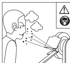
Material and dust flying towards the operator's eyes and body. Use eye protection and an anti-dust mask.
