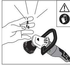
Risk of cutting and abrasion. Keep safety distance from the working area, the abrasive elements, and do not touch any of the moving parts. Always wear protective gloves.
