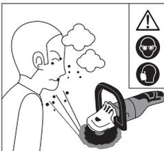
Material and sparks flying towards the operator's eyes and body. Use eye protection and an anti-dust mask.
