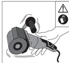
Danger of high vibrations. Put on the anti-vibration gloves. Take rest breaks during processing.
